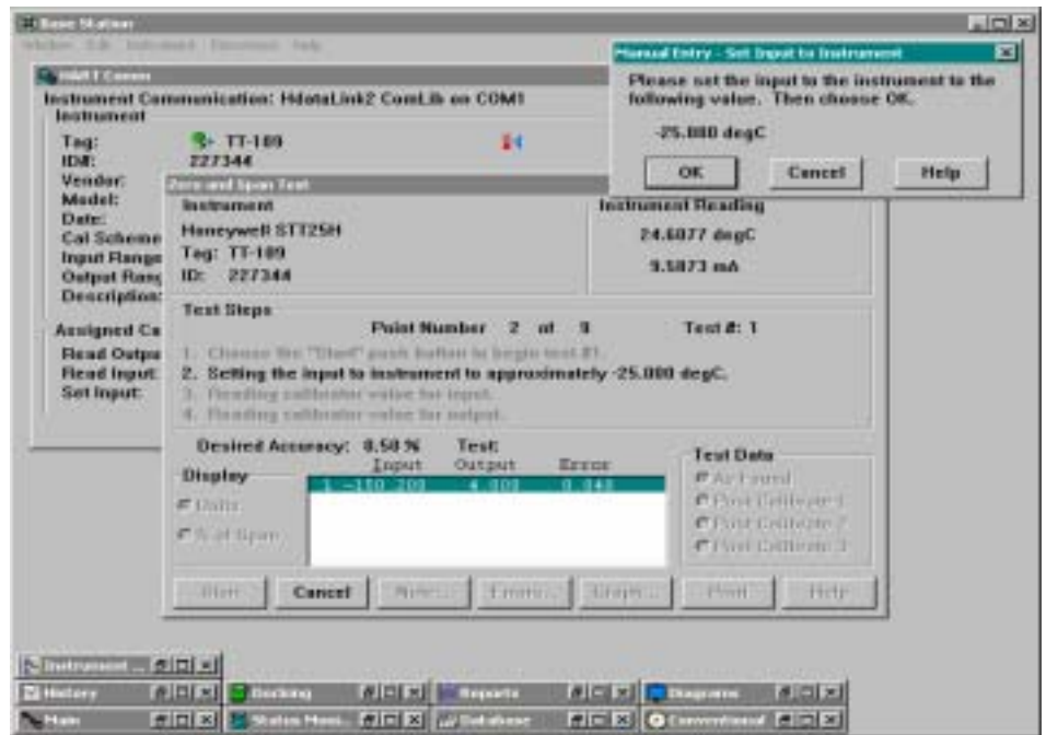
Use the HART Comm window to perform computer guided multi-point tests
